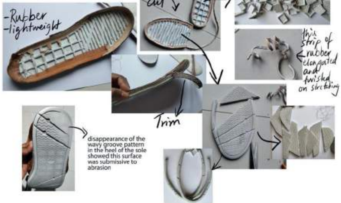
Figure 10. 'Robotically' deconstructing the sole. Image: Aysh Balakumar
