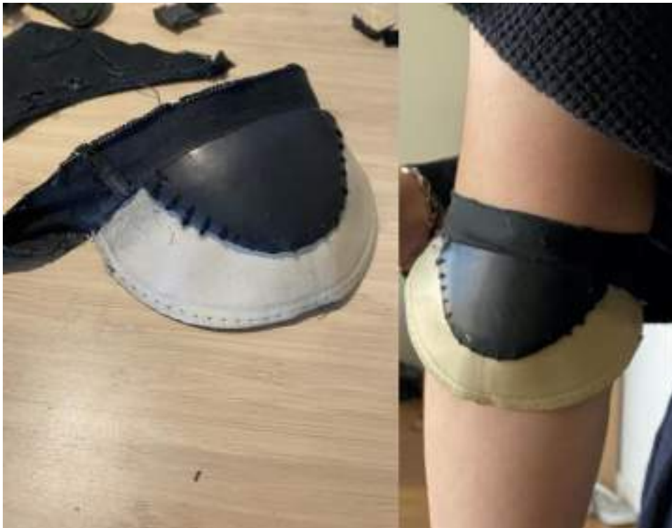
Figure 6. Heel counter, toe cap and canvas upper. Image: Madsy McInnes-Smith
